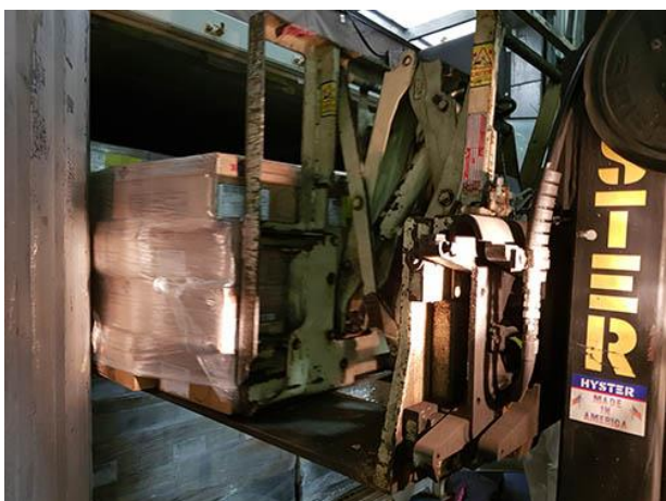
Slip sheet pallets be unloaded. Total of 24 pallets.
