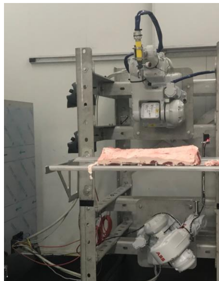
Figure 2: Two-arm robot arrangement in plant trials.
