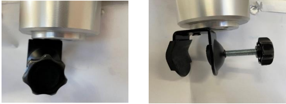
Figure 28: Brackets used to hold the trimmer in place
