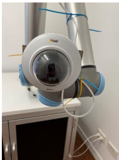
Figure 23- Installation of roll-face Network Camera
