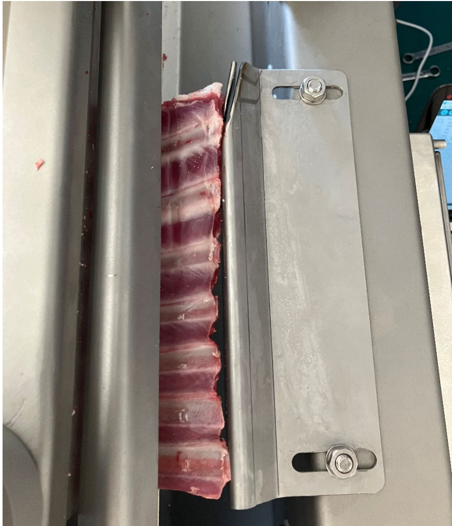
Figure 15: Cut line of rack bones is often not straight which requires the tip sensor to be offset from actual tip
