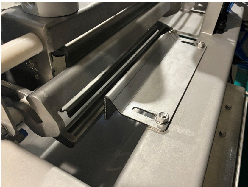
Figure 7: Frenching length adjustment backstop
