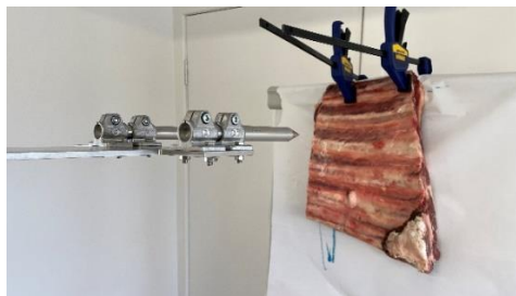
Figure 12 - Setup for short rib marking trials
