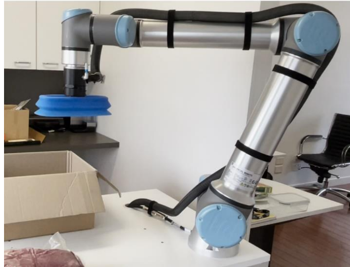
Figure 16 - Collaborative Robot with Gripper Installed
