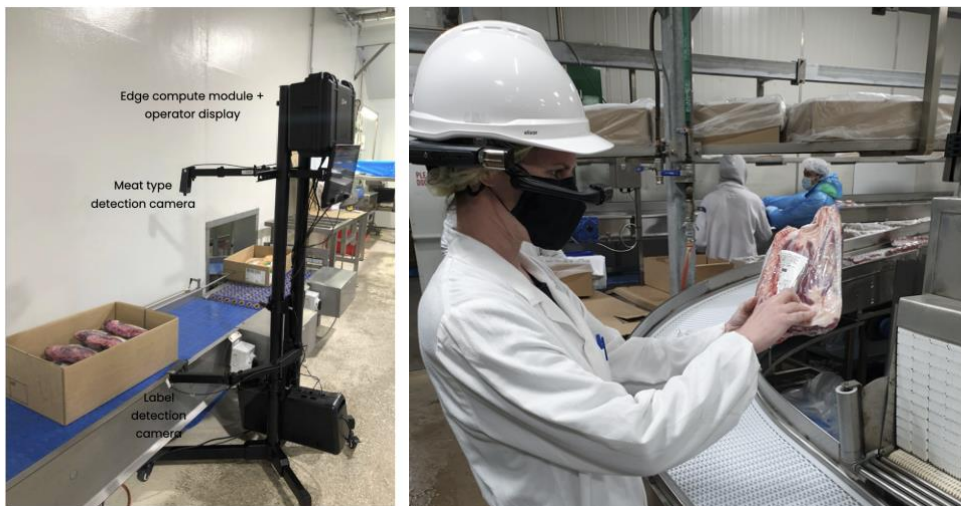
Figure 1: (Left) BLV rig in operation at a VIC meat processing facility, (Right) Remote inspection using smart glasses
