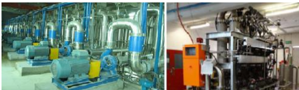
Figure 2: Ceramic membrane plant using Jiuwu membranes, China ( http://jiuwu.cphi-online.com/Product/16541/Ceramic_membrane_machine ) (left) and metallic membrane plant using AMS membranes, Australia ( http://www.ams100.com/ )
