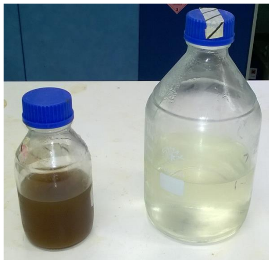
Figure 27: Appearance of samples taken from membrane distillation including concentrate (left) and permeate (right). Some feed contaminated the permeate due to fat contamination on the membrane.
