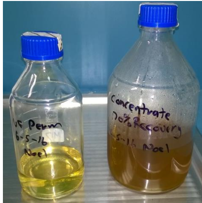
Figure 24: Appearance of samples taken from UF including permeate (left) and concentrate (right).
