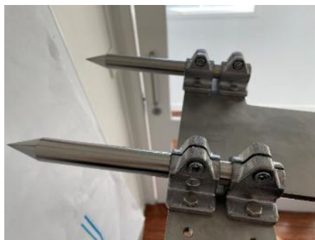
Figure 44: Scribe tool setup in bracket attached to robot rollface
