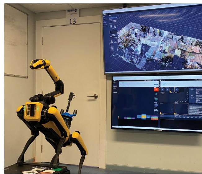
Boston Dynamics Spot Enterprise Robot – an automated guided vehicle with articulated legs.
