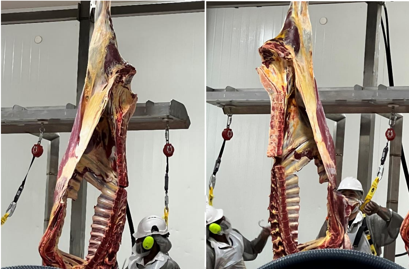
Figure 2: Prototype 1 installed into the boning room on platform. Inertia reels extending as movement occurs.
