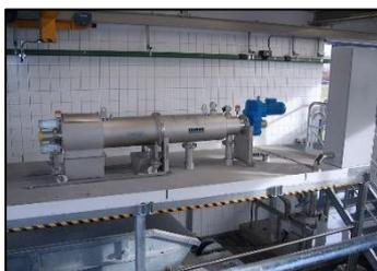
**Screw presses** comprise of a rotating screw in a compression barrel, fitted at the inlet end, with a slotted screen for initial dewatering. Compressed solids form a 'plug' at the discharge end, against which the incoming solids are compressed by the action of the screw and dewatered.
