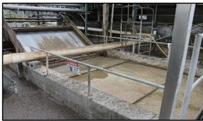
**Savealls** are large settling tanks. Fats separate and float to the top and heavier solids sink. Surface scrapers tease the floating fat off the liquid surface. Sometimes base scrapers remove solids in a similar manner.
