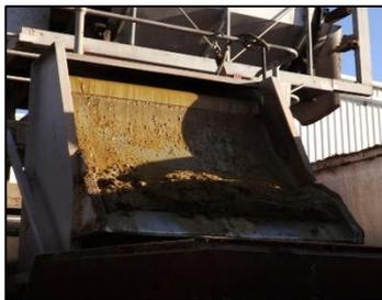
**Static screens** are usually a vertical bow shaped wedge-wire screen. Most of the liquid drains through the screen while the solids collect at the base before discharge.
