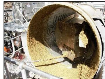
**Rotary screens** use a rotating horizontal cylindrical screen. The solids move to the opposite end of the rotating cylinder, where it discharges.
